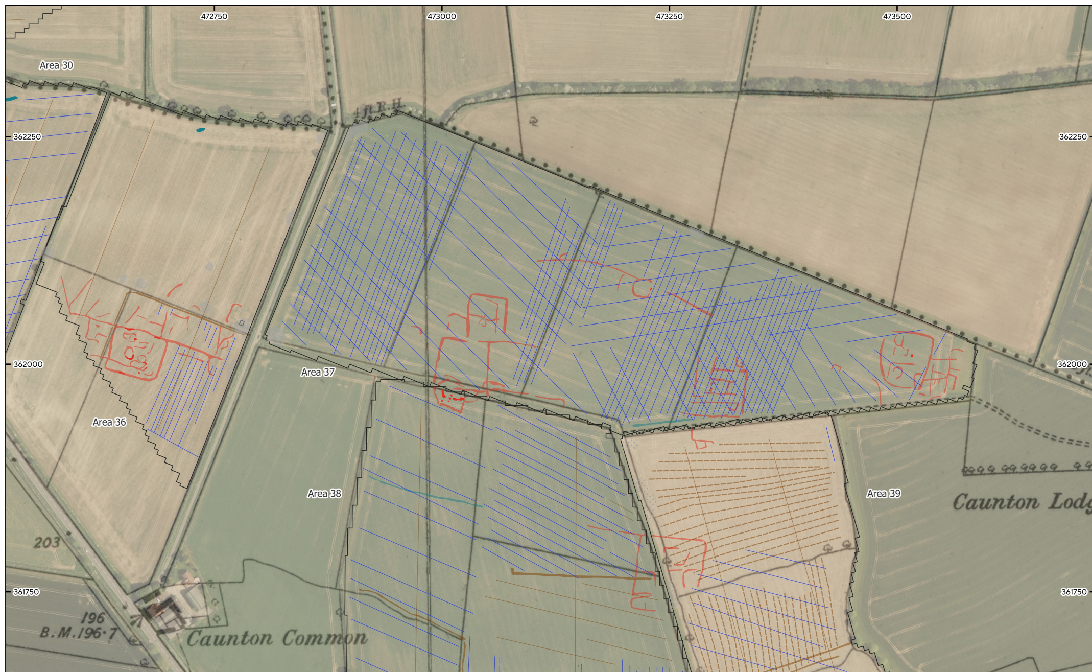
MSSK1838 - Great North Road Solar Farm, Staythorpe Figure 26 - Magnetic Interpretation over Historical Mapping (Areas 30, 36, 37, 38, & 39) 1:3,000 @ A3 © Magnitude Surveys 2025 Contains Ordnance Survey data © Crown Copyright and database right 2025
