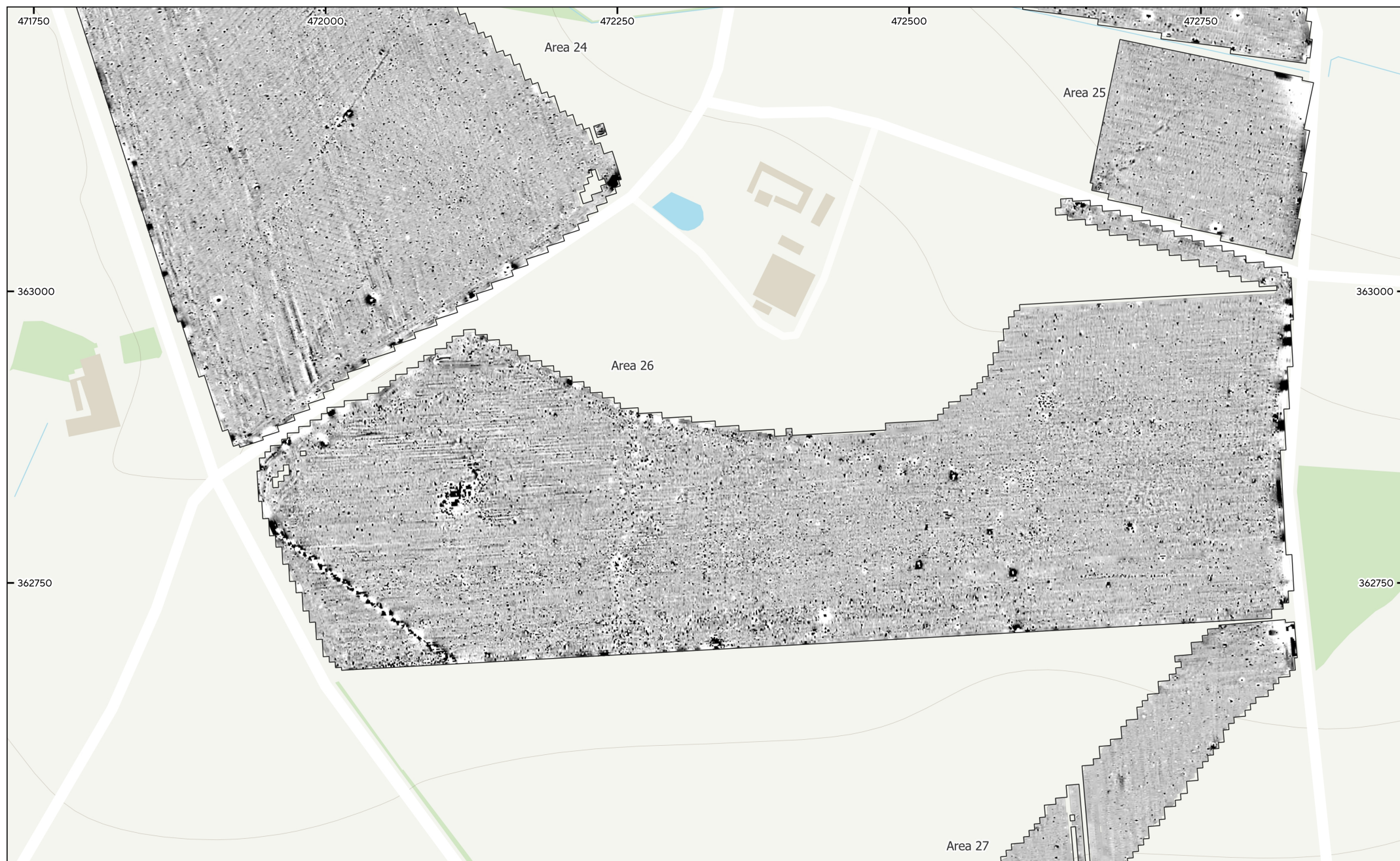
MSSK1838 - Great North Road Solar Farm, Staythorpe Figure 21 - Magnetic Gradient (Areas 24, 25, 26, & 27) 1:3,000 @ A3 © Magnitude Surveys 2025 Contains Ordnance Survey data © Crown Copyright and database right 2025
